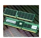
active (primary) until the failing DIMM is replaced. Mirroring can be accomplished with multiples of *four* DIMMs (one pair per memory channel).
