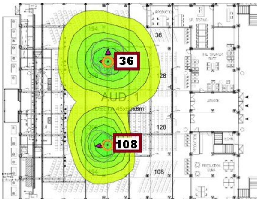
Figure 41: Example using "E/P" version to create two macro cells can be supported
