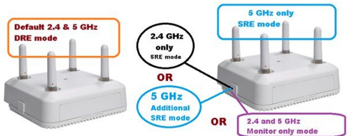
Figure 36: Antenna control (default) and with smart antenna connector installed
